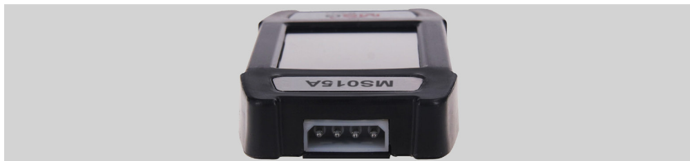
Figure 2. Diagnostic cable connection port
