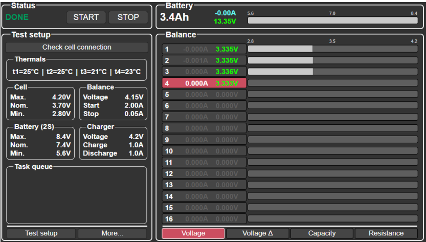
Figure 11. Example: missing “crocodile” clamp on cell 4
