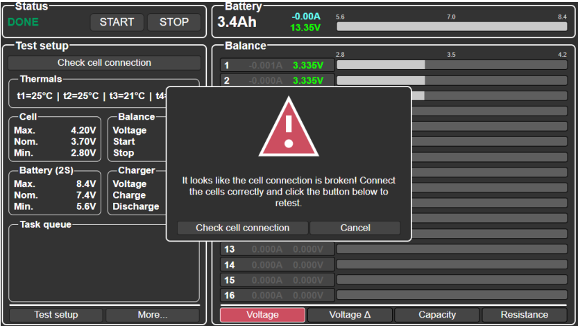
Figure 12. Example: missing clamp(s) on the edge cells of the battery
