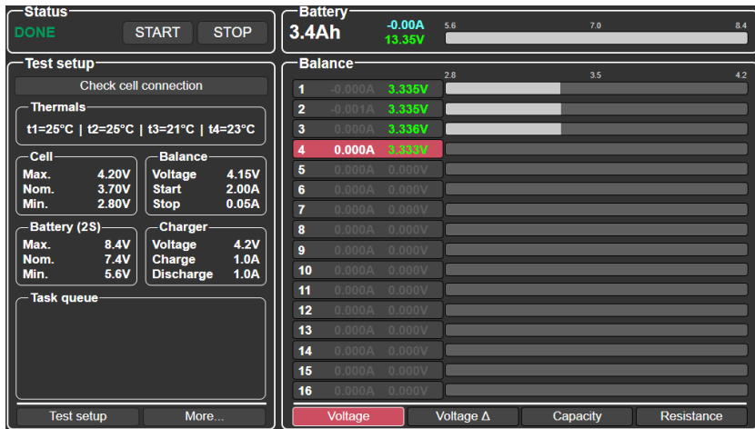
Figure 11. Example: missing “crocodile” clamp on cell 4
