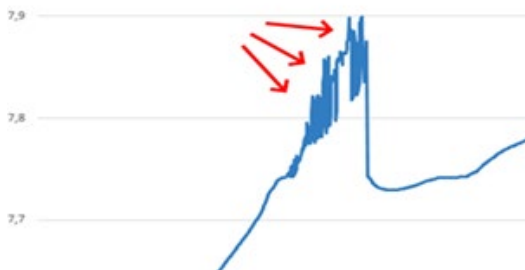
Figure 16. Voltage change on the module with the not proper connection of clamps
