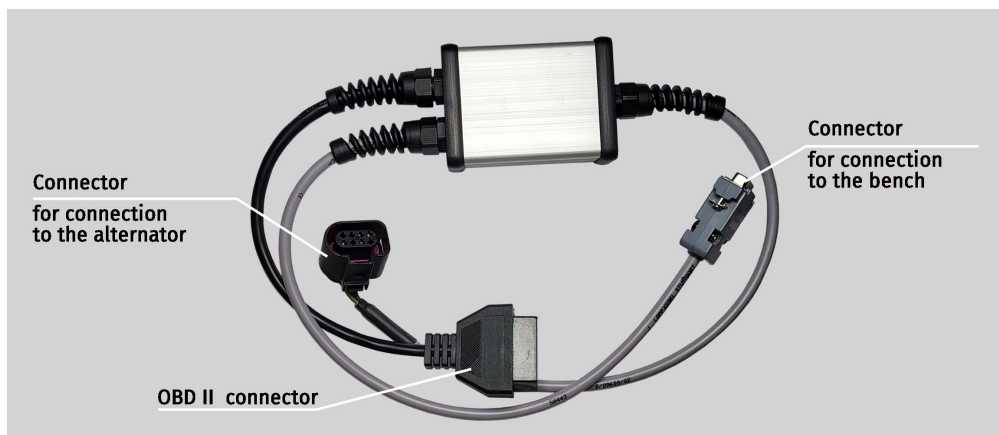
Figure 8. Cable for testing 48 V belt starter-generators
