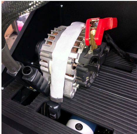
Figure 16. Connection of Power Wires to the Alternator
