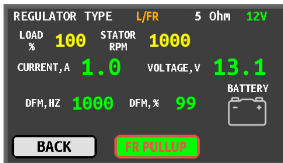
Figure 10 – Diagnostic screen for 12/24V voltage regulators of L/FR type
