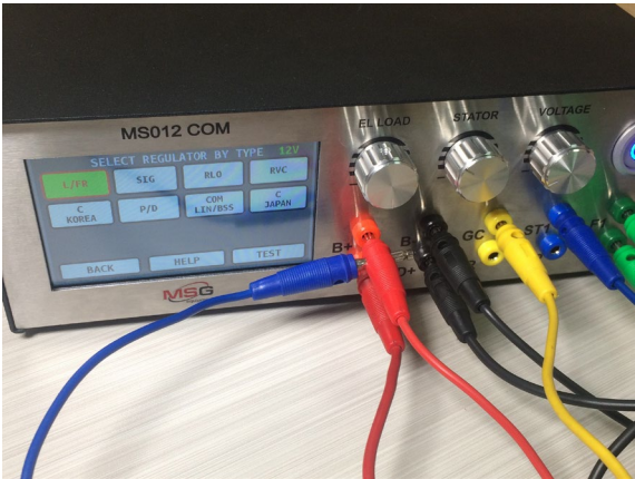
Figure 19 – Connection of additional cable B+
