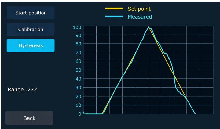
Figure 17. Holset actuator programming screen
