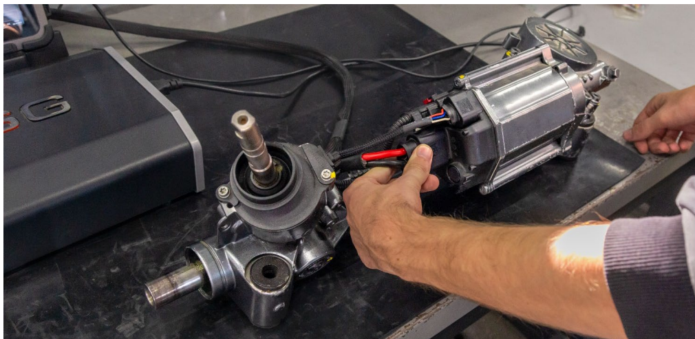
Figure 3. Connecting an EPS unit to the tester
