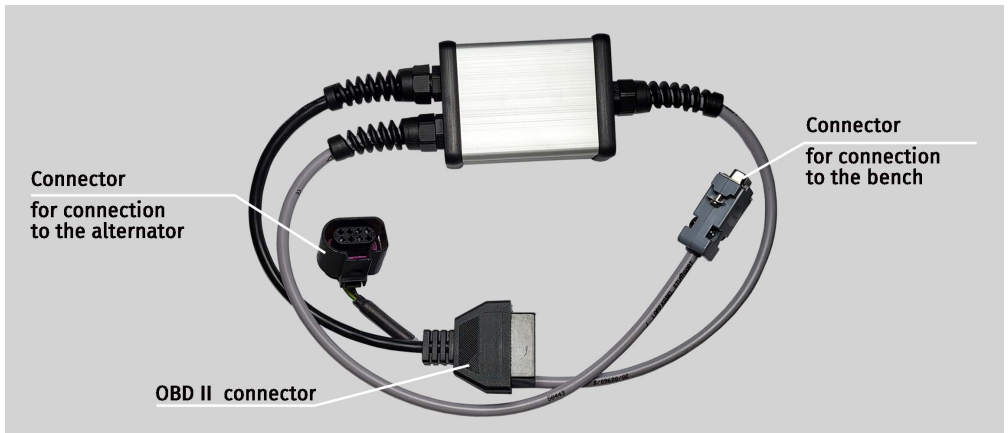
Figure 8. Cable for testing 48 V belt starter-generators
