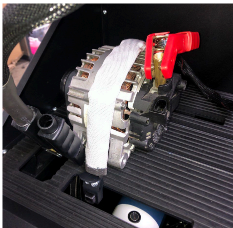
Figure 16. Connection of Power Wires to the Alternator
