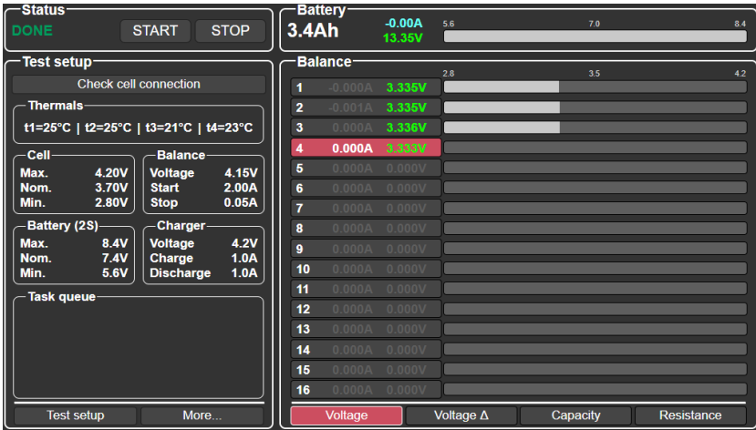
Figure 11. Example: missing “crocodile” clamp on cell 4
