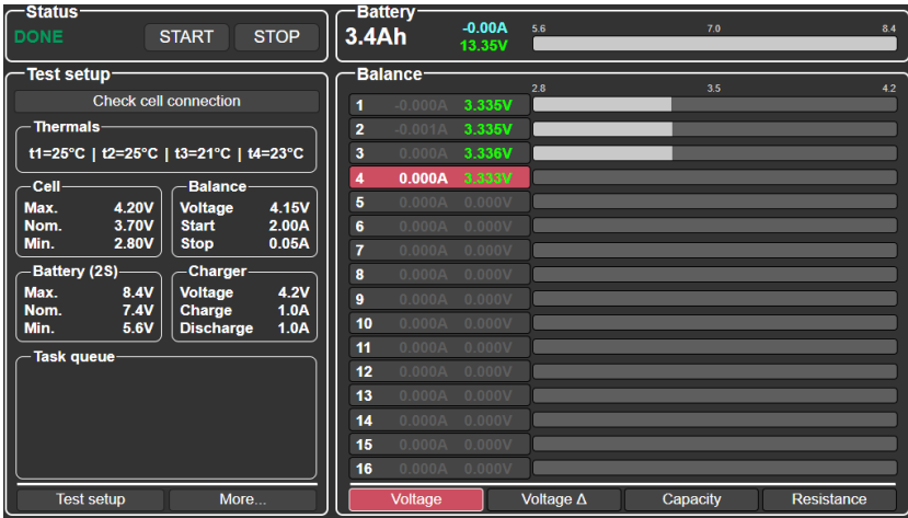
Figure 11. Example: missing “crocodile” clamp on cell 4
