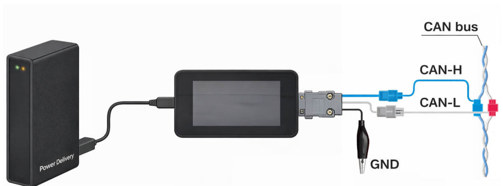
Figure 33. Example of connection to the CAN bus with power supplied from a portable battery
