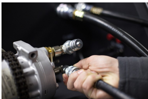
Figure 25. Connection of the LP and HP lines to a compressor
