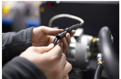
Figure 27. Connection of control wires to a compressor
