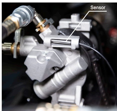
Figure 29. Position of a contact temperature sensor
