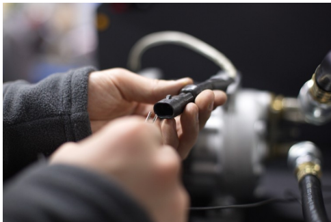
Figure 27. Connection of control wires to a compressor
