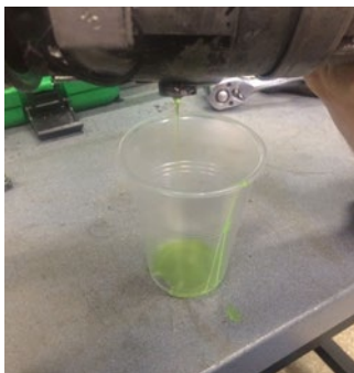
Figure 21. Monitoring of compressor oil condition
