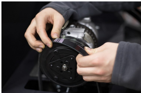
Figure 24. Adjusting the belt and checking its tightness
