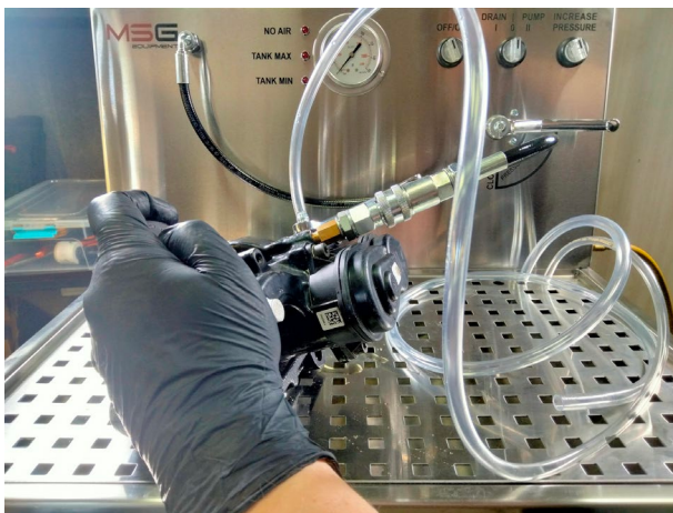
Figure 11. Connected PVC tube for pumping
