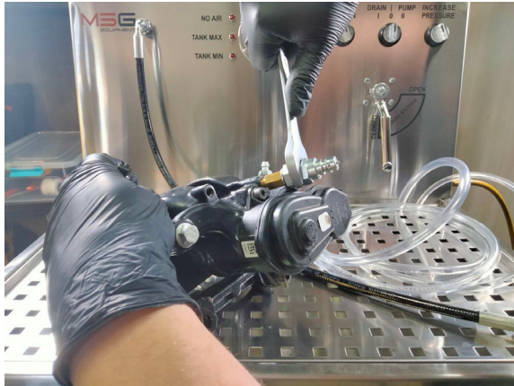
Figure 9. Installing the coupling with adapter on the caliper
