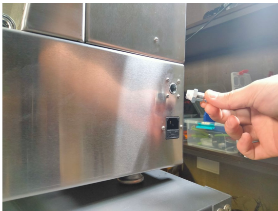
Figure 3. Mounting the quick disconnect fitting for connecting the compressed air supply
