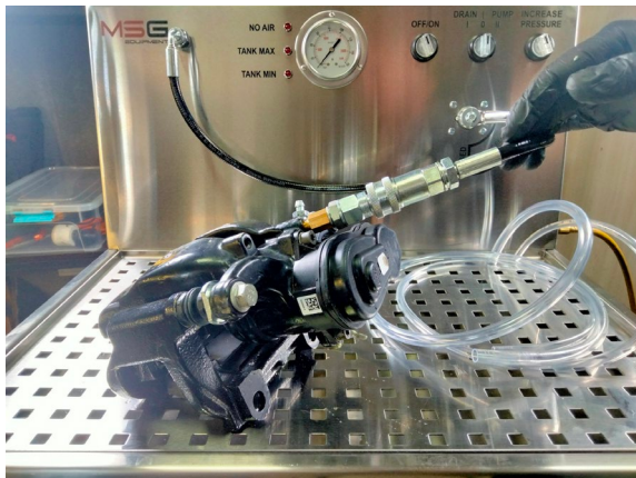
Figure 10. Connecting the high-pressure hose
