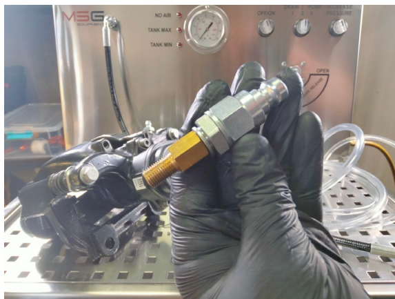
Figure 8. Connector and adapter matched to caliper threads
