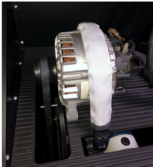
Figure 14. Installation and Fixation of the Alternator on the Bench
