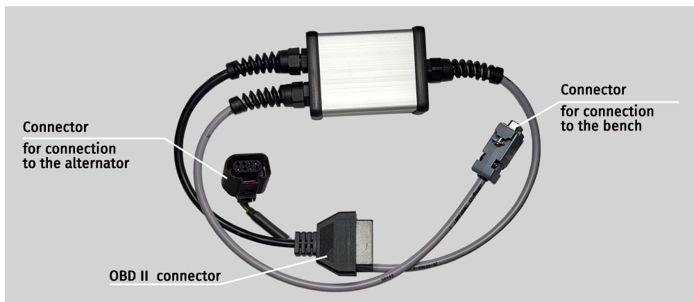
Figure 8. Cable for testing 48 V belt starter-generators
