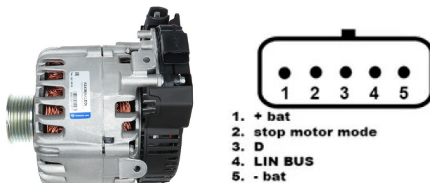
Figure 13. Valeo IST60C017 alternator and terminal designations in the socket
