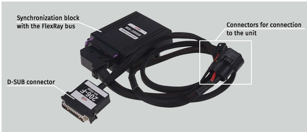
Figure 7. Specialized FlexRay cable
