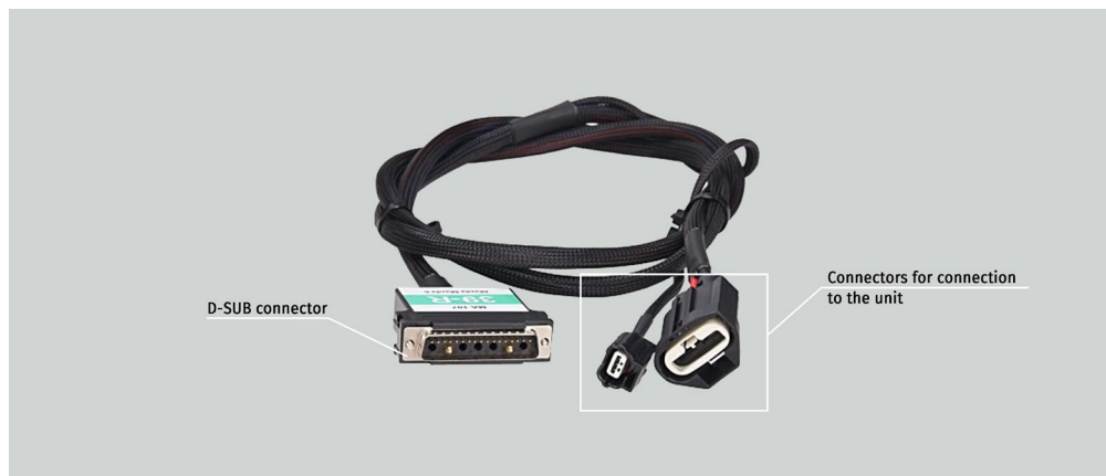
Figure 6. Specialized CAN cable
