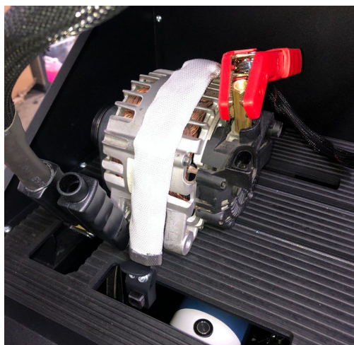
Figure 16. Connection of Power Wires to the Alternator
