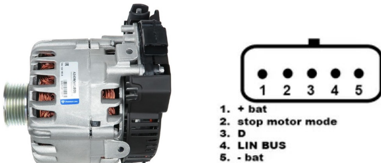
Figure 25. Valeo IST60C017: marking of terminal pins
