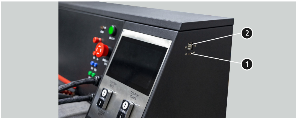
Figure 3. Connectors on the side panel of the bench: 1 – HDMI; 2 – USB
