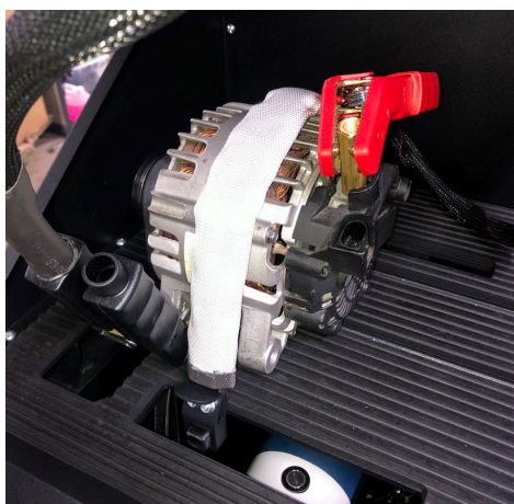
Figure 13. Connection of Power Wires to the Alternator
