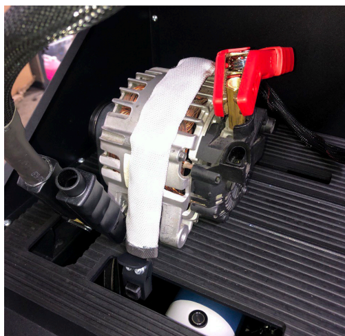
Figure 16. Connection of Power Wires to the Alternator
