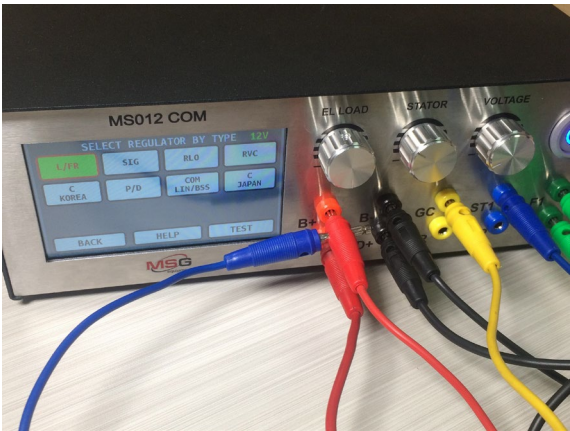
Figure 19 – Connection of additional cable B+
