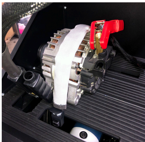
Figure 16. Connection of Power Wires to the Alternator
