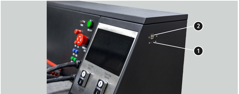
Figure 3. Connectors on the side panel of the bench: 1 – HDMI; 2 – USB
