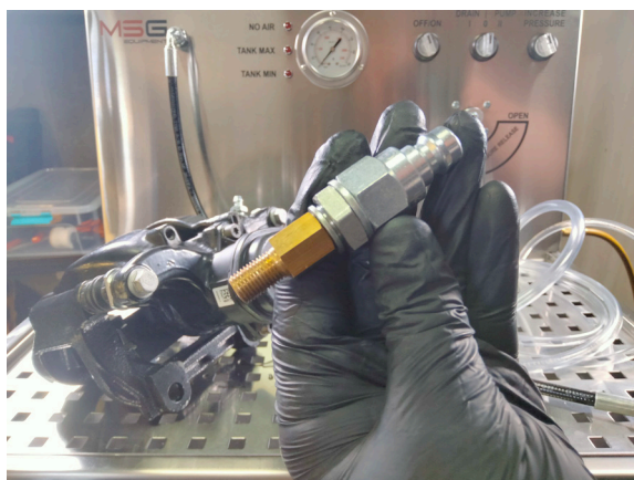
Figure 8. Connector and adapter matched to caliper threads
