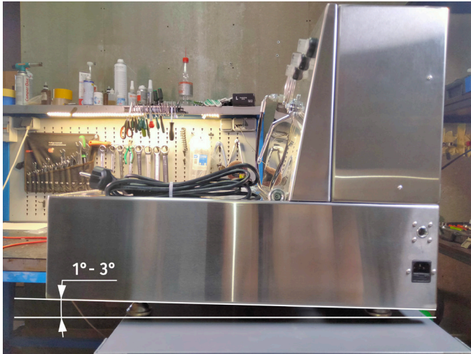
Figure 2. Correct position of the bench
