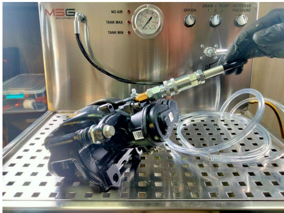
Figure 10. Connecting the high-pressure hose
