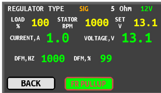
Figure 11 – Diagnostic screen for voltage regulators of SIG and P-D types
