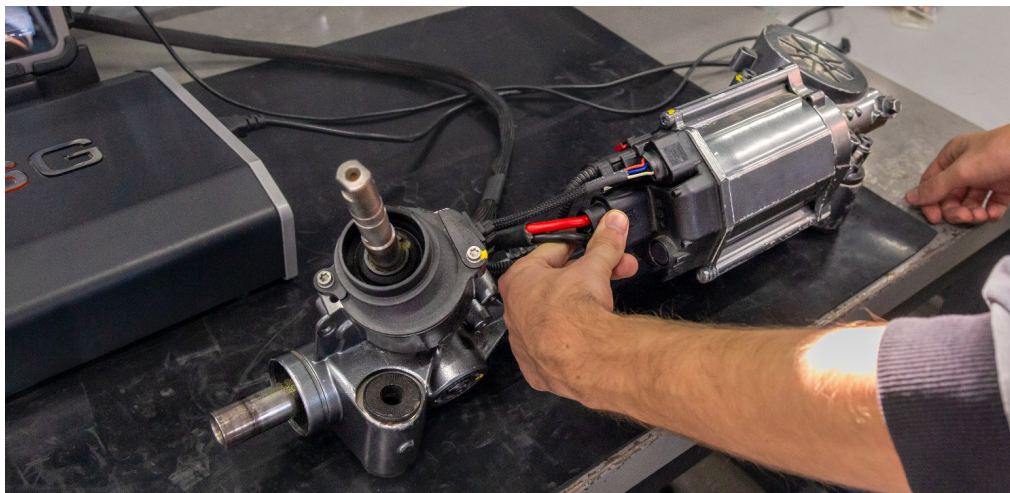
Figure 3. Connecting the EPS unit to the tester
